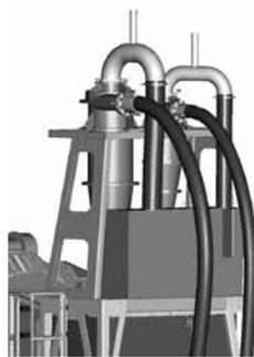
Specialized rubber lined sealed slurry transfer pipe complete with heavy duty clamps
