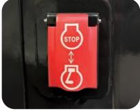
Secondary engine shutdown switch
