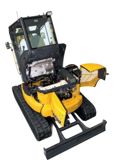
Rear bonnets for quick engine checks, simple inspections, cleaning of the radiators and easy access to the battery
